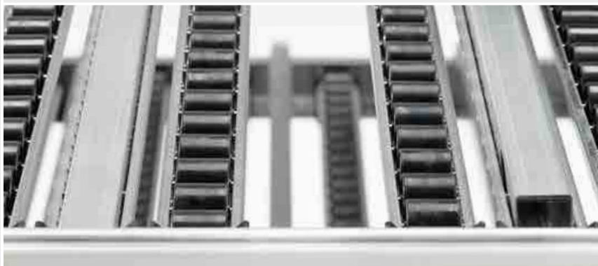
Retracting or extending the dividing rail enables containers with different dimensions to be mixed on one level
