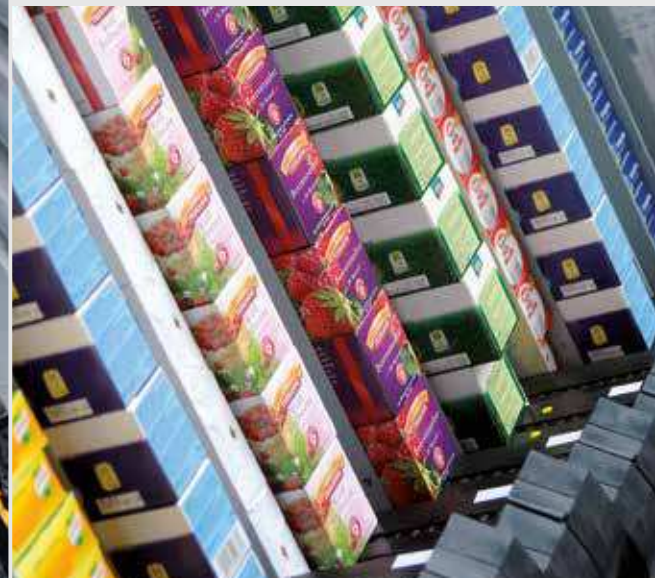
▲ Filling point ► Collecting belt ▼ S-Pemat channels with one ejector per channel
