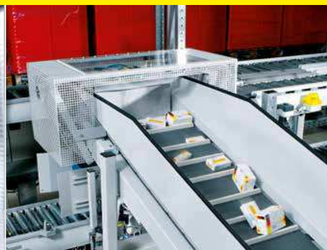
▲ Filling point ► Collecting belt ▼ S-Pemat channels with one ejector per channel
